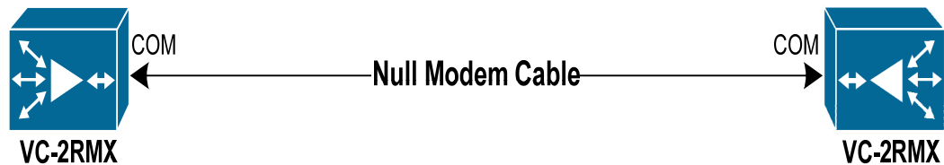
Figure 4-2: Com to Com Null Modem Direction Connection
